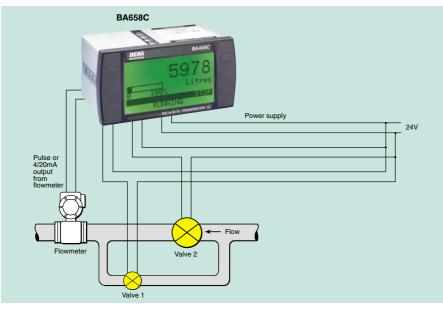
**The BA658C** is a second-generation, general-purpose flow batch controller that supersedes the successful BA550P and BA550C. This controller is ideal for accurately dispensing liquids, solids or components and despite its sophisticated control functions, it remains very easy to use and configure.
